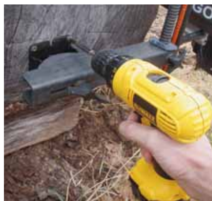
Attaching the bracket to the end of the log. The Big Mill uses a bracket bolted on to each end of the log to hold the guide rail. These must be leveled at both ends so that the chain saw cuts a straight line.
