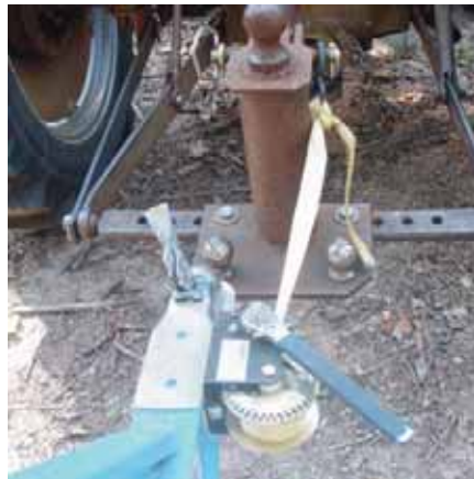
Hitching the arch to the tractor was frustrating until I mounted a second winch to the hitch to pull the arch up to the tractor.
