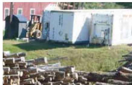
The two firewood kilns flank a larger trailer box used as a storage barn. The Central Boiler outdoor furnace is seen on the left.
