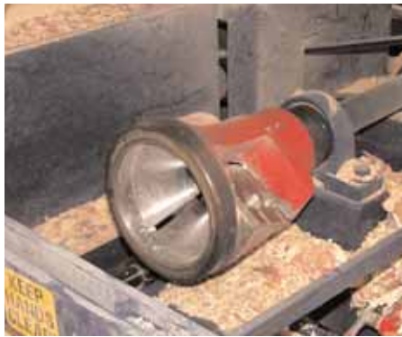
The tenon cutter has two straight taper cutters that quickly unbolt for sharpening.
