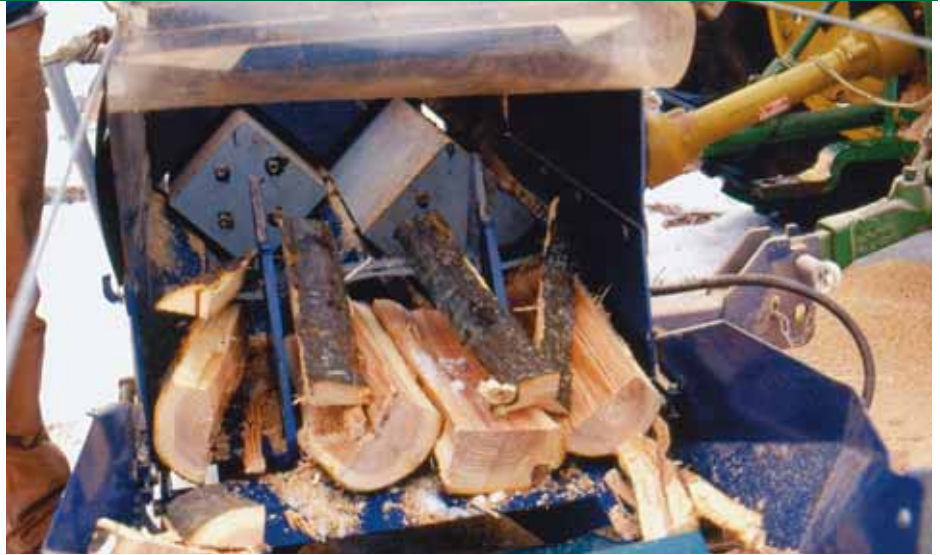
The two splitting cylinders work alternately as the wood is dropped first into one empty trough and then into the other. Here we see the two splitting cylinders and the wedge.
