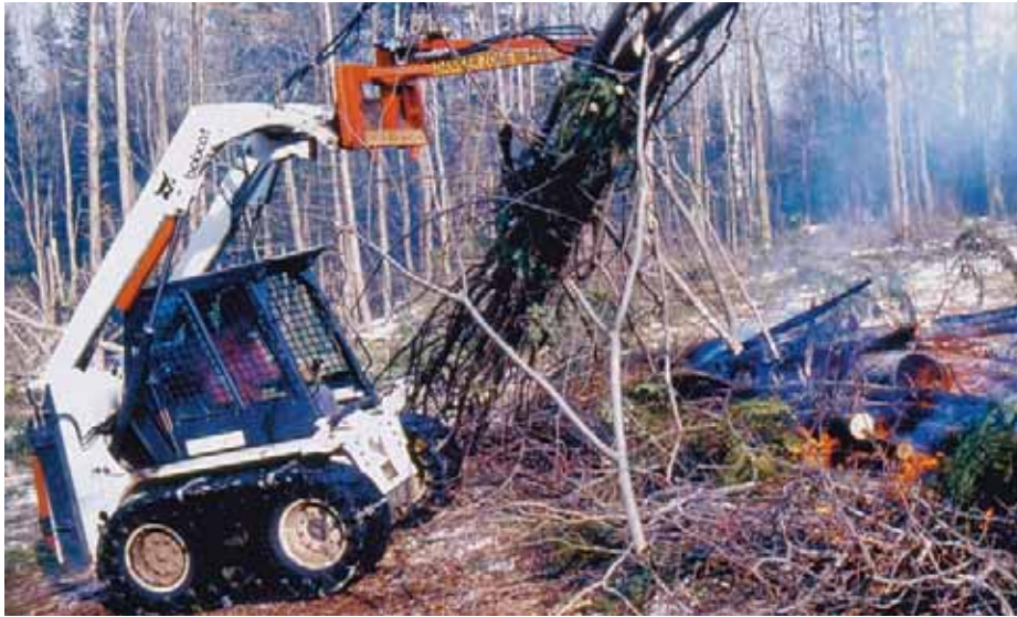
The skid-steer grapple is perfect for piling brush and small tree stems on a brush fire.
