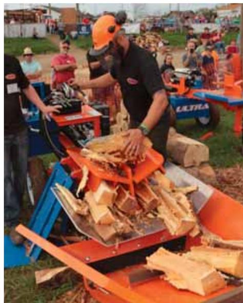
hydraulic ram can handle pieces up to 24 inches in length. When asked about the maximum diameter the Ultra can handle, Andrew replied that he had split logs over 40 inches in diameter with no problem. "If you can get it on the splitter, it can handle it," he said. The extra push from the 2-stage hydraulic pump kicks in for crotches and other unusually tough pieces.
