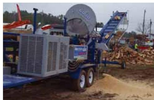
tion to the faster cutting rate, the inserted-tooth blade requires less sharpening and individual teeth can be quickly replaced, if necessary. “In the 13,000 hours we've run the machines, we've never touched a tooth yet,” he noted. “The only maintenance has been an oil change every 250 hours.”
